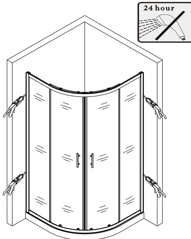
Apply some silicone on the outside edge of the shower enclosure (between the wall profiles and wall and between the frame and the tray) to enhance waterproof. After installation, it needs 24hours for silicone to dry before being put into use.
