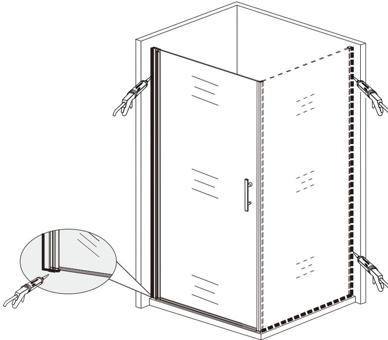
Apply some silicone on the outside edge of the shower enclosure (between the wall profiles and wall and between the frame and the tray) to enhance waterproof. After installation, it needs 24hours for silicone to dry before being put into use.
