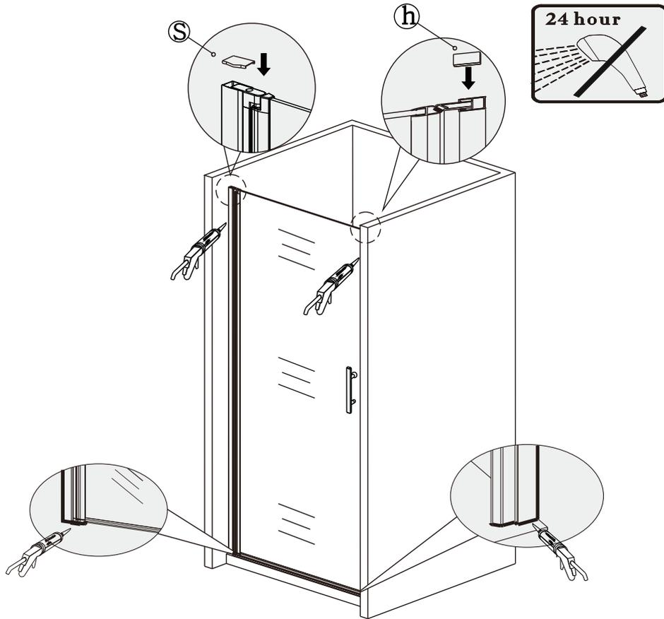
Apply some silicone on the outside edge of the shower enclosure (between the wall profiles and wall and between the frame and the tray) to enhance waterproof. After installation, it needs 24hours for silicone to dry before being put into use.
