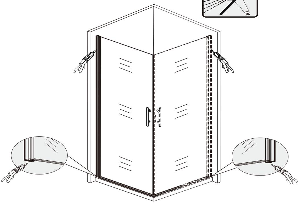
Apply some silicone on the outside edge of the shower enclosure (between the wall profiles and wall and between the frame and the tray) to enhance waterproof. After installation, it needs 24hours for silicone to dry before being put into use.
